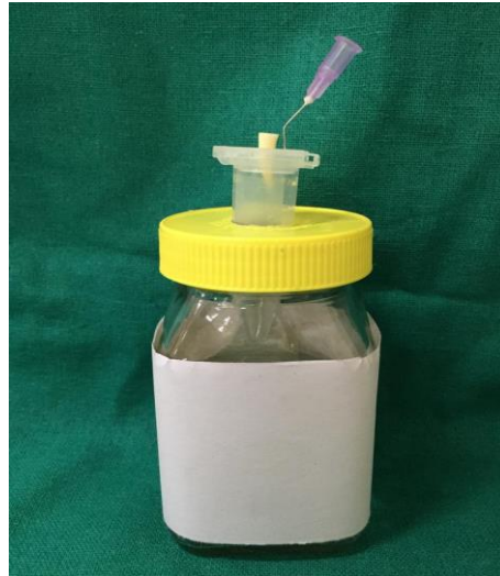
Setup for debris Collection (Eppendorf tube with mounted tooth and 27-G needle)
