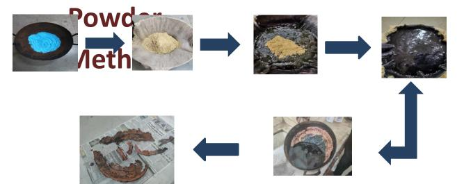
**Figure 2: Extraction of Pure Copper** Figure 2 shows the Extraction of Pure Copper
