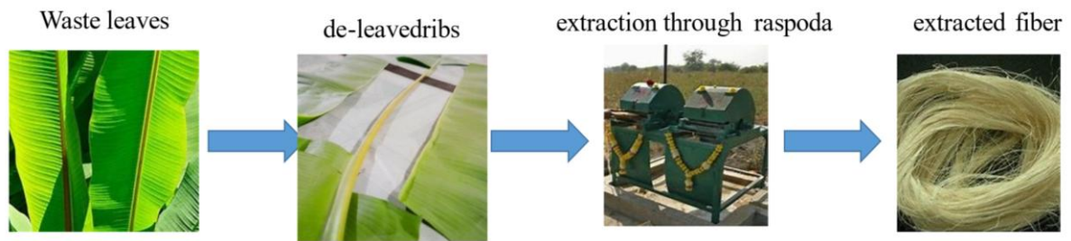
Fig.2 Procedure for the extraction of fiber from leaves
