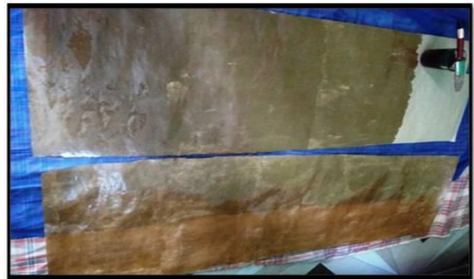
Fig. 3. Layering of fresh paper with additives (WSR, DSR and Apcotex) during day time
