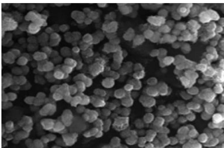
**Figures 4: Morphological of polymeric microparticles**
