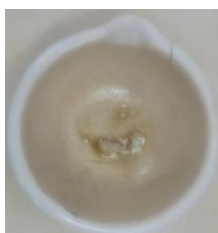
Fig.2. Pure Silver post drying in Muffle Furnace
