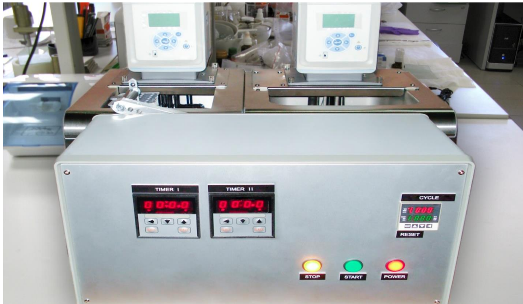
Figure 2. Thermal cycling device.
