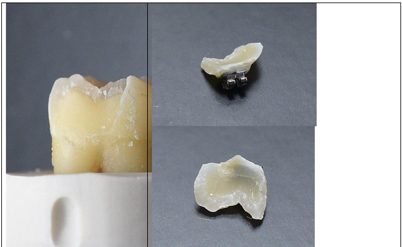
Figure 6 – Destruction of a tooth sample along the enamel-dentin boundary
