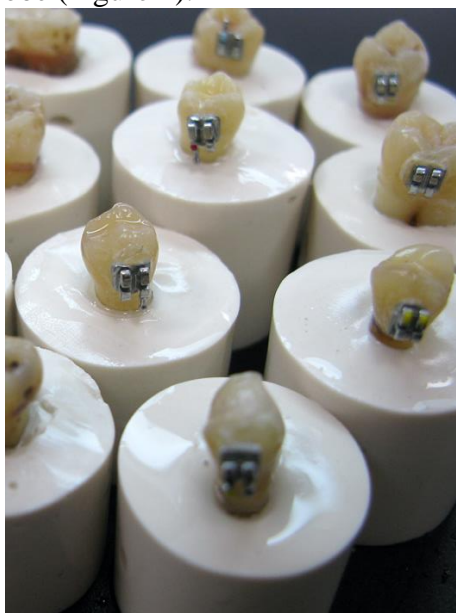
Figure 1 – Samples of metal bracket systems prepared for research
