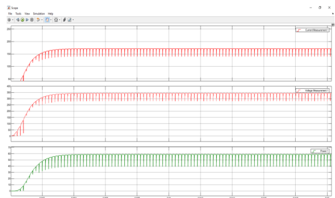
Fig9. Output Current, Voltage, Power at MPP
