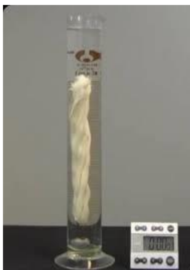
Figure 3. Wetting efficiency by Draves test
