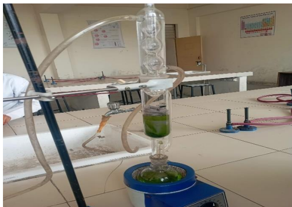
Fig No.3: Soxhlet assembly (extraction)
