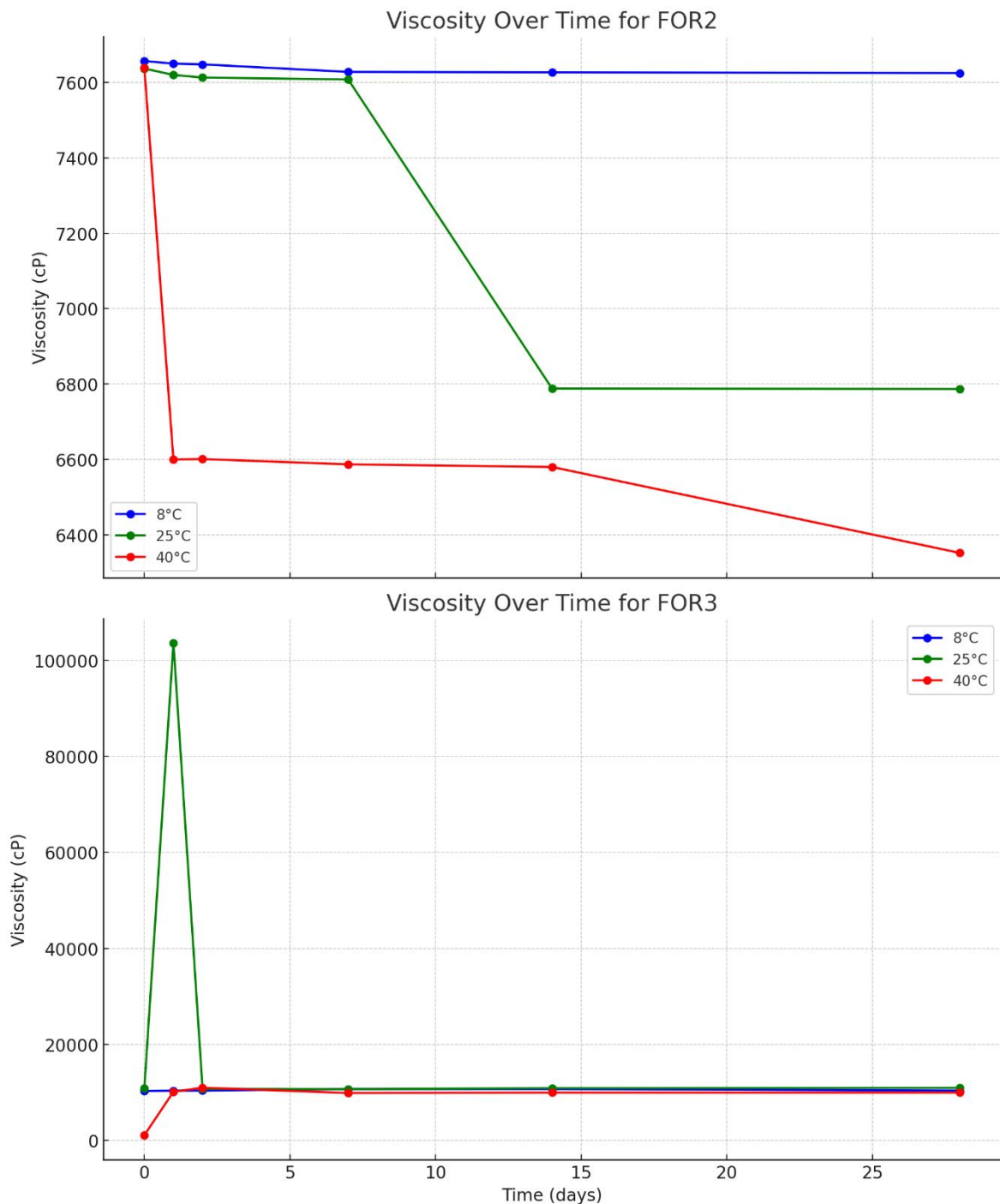
Figure 4. The viscosities of the formulations (FOR2 and FOR3) were shown as centipoise at different times and temperatures.
