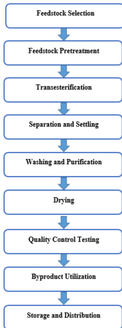
Figure.3.1 Biodiesel production process
