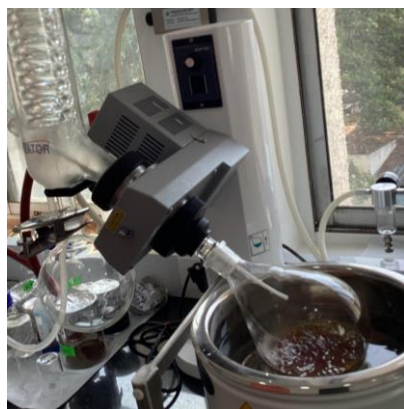
Figure 4 depicts the process of flash evaporation of anthocyanin at 34 degree Celsius
