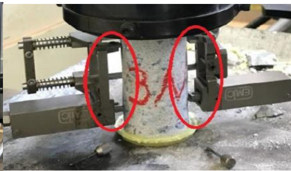
Fig. 6. Modulus of elasticity test
