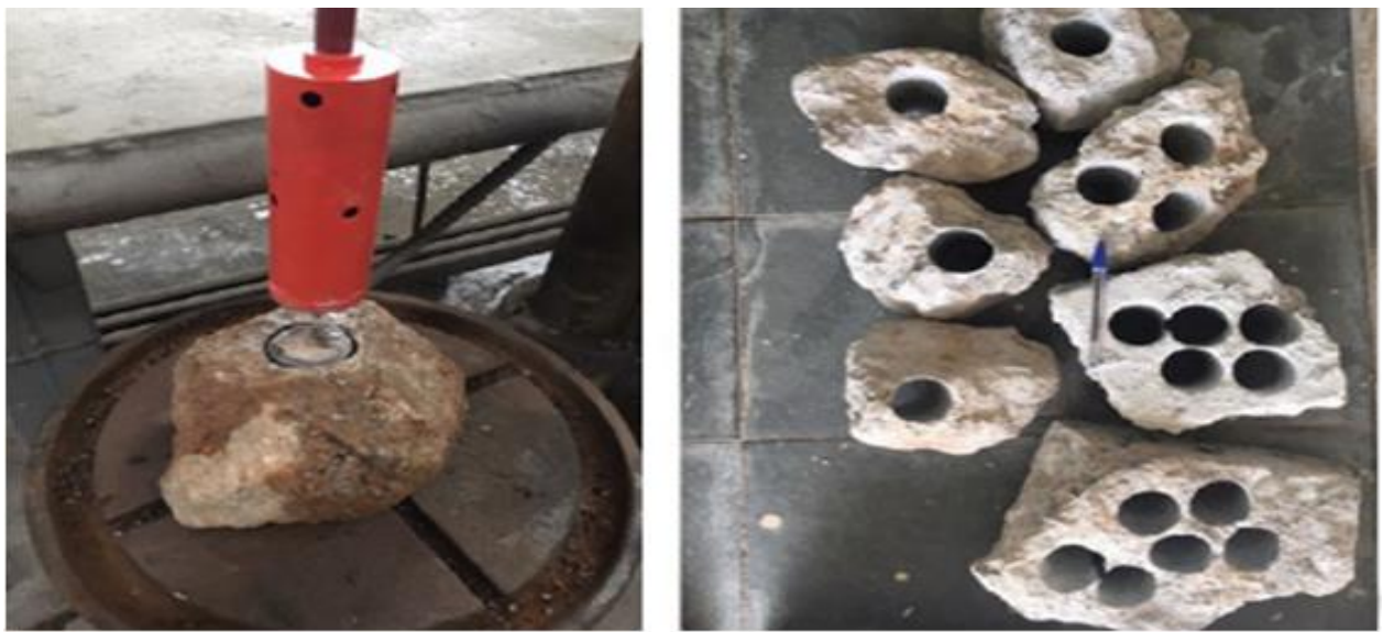
Fig. 1. Extraction of Specimens
