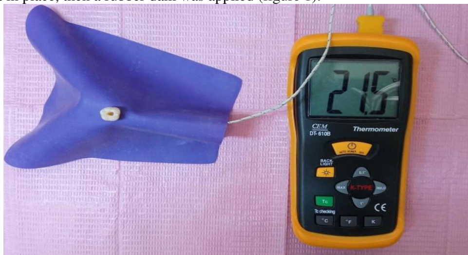
Figure 1: showing the tooth attached to the vice and the thermocouple and connected to the thermometer and rubber dam was applied
