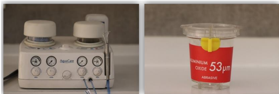
Figure 11. The airborne particle abrasion on the specimen using 29 Mm grain sized Al_2O_3 particles the performance made in circular movements at a standoff distance of 1 cm at angulation 45 degree with 2.8 bar pressure for 15s.
