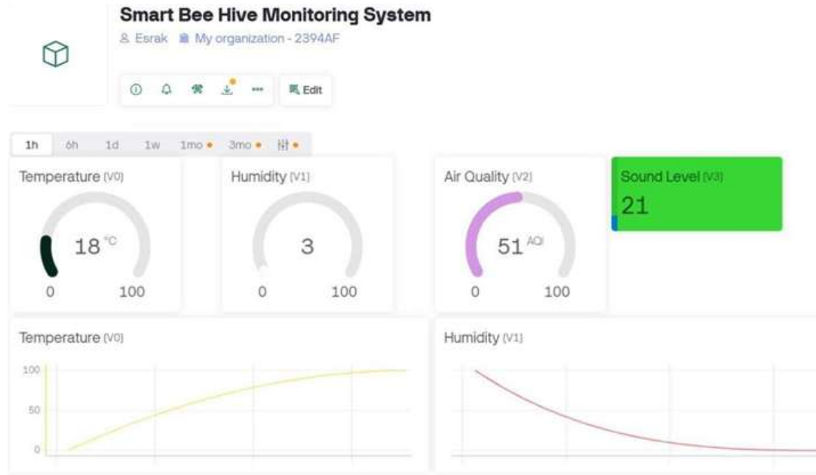
Fig. 7: Dashboard of Sensor data on Blynk. One incident data of Bee hive monitoring system.
