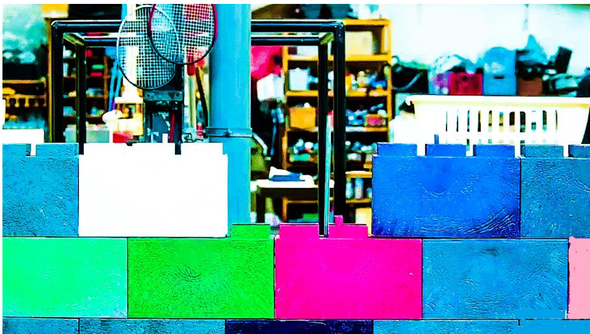
Figure:2 Plastic trash has been used to create lightweight bricks and blocks.
