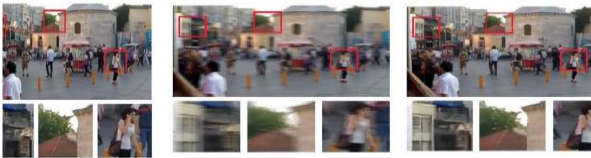
Figure 4 . Shows the images for deblurring in which (A) Shows the original image, (B) Shows the image that is being blurred due to Gaussian noise, and (C) Shows the image generated after the DeblurGAN algorithm [20]
