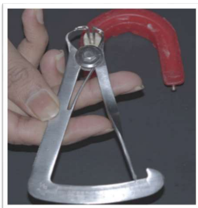
Figure 3: Figure representing the working methodology of the novel endodontic caliper for making the interorificial measurements in the given samples
