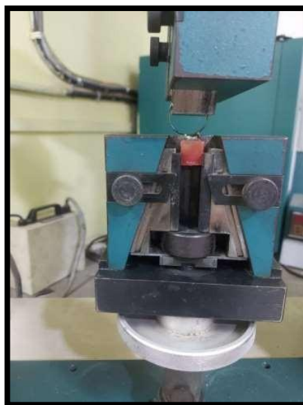
Figure 1: Specimen undergoing bond strength testing in the universal testing machine.
