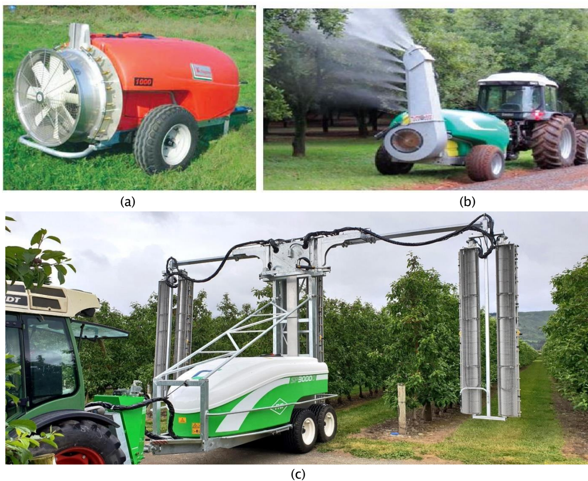
Figure 3. Air-assisted sprayers; a) Axial fan type, b) Centrifugal fan type, c) Crossflow/ tangential fan type
