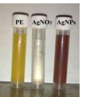
the reduction of silver ions. nanoparticles exhibit aqueous solution due to plasmon vibrations in silver appearances of yellowishbrown colour (Fig. 1) in the reaction vessels suggest the formation of silver nanoparticles (SNPs)<sup>11</sup>.
