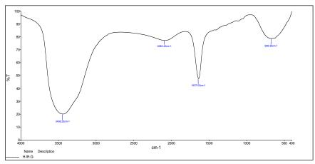
Figure 3 FTIR analysis of silver nanoparticles synthesized by treating 1mM aqueous AgNO<sub>3</sub> solution with *Sansevieria roxburghiana* leaf extract.
