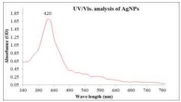
Figure 2 UV-Vis absorption spectrum of silver nanoparticles synthesized by Sansevieria roxburghiana leaf extract after 5 hrs.
