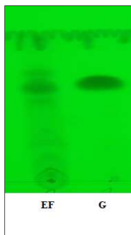
Figure: Gallic acid (G) & ethyl acetate (EF) fractions are separated using thin layer chromatography using Silica Gel GF254. Created with the Solvent System (Chloroform: Acetone: Formic Acid (75: 16.5: 8.5)), UV Light 254 nm Detection.
