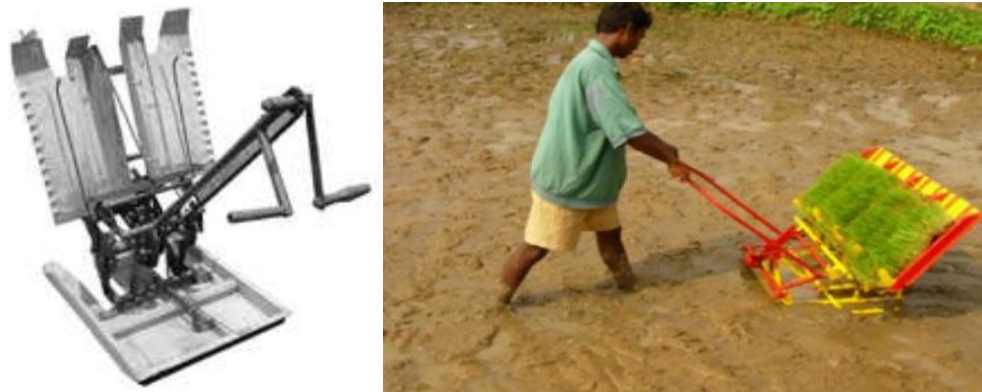
Figure 9. Manually operated, hand-cranked rice transplanter walking backward type (left) and walking forward type(right)
