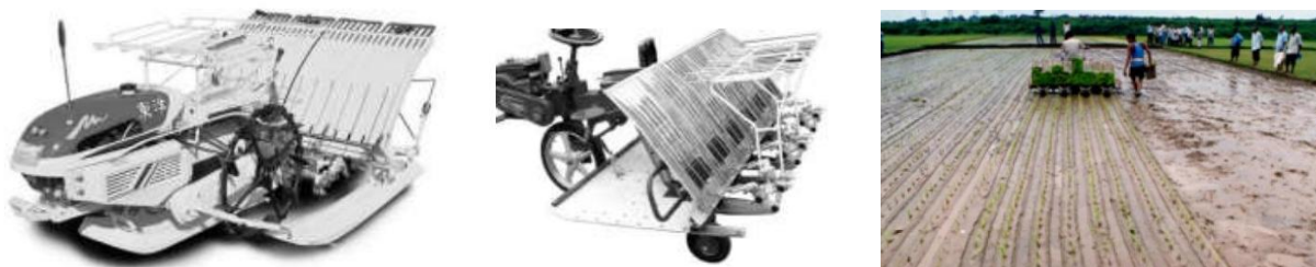
Figure 10. Walking behind (left) and Self-propelled paddy transplanter, (middle), Self-Propelled at Operation, (right side) (source: Dixit and Khan, 2011).
