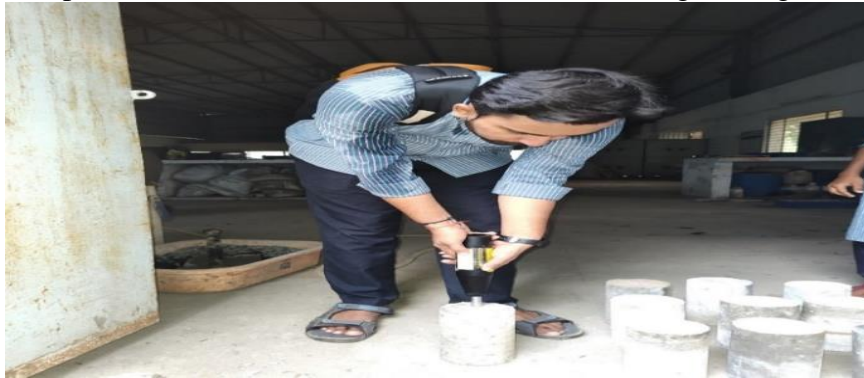
Fig 4 strength test using rebound hammer
