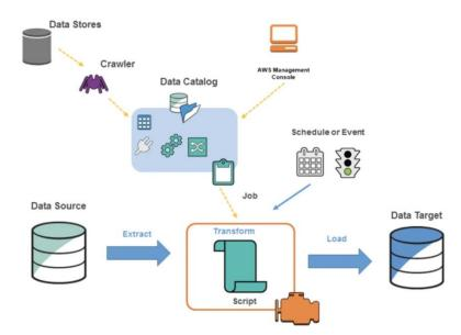
Fig.1. Diagram showing the working principal of AWS Glue
