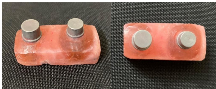
Fig. 1. Steel abutments in an acrylic block
