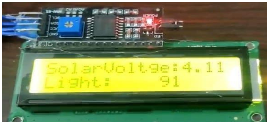
Fig. 8. Display of output voltage readings and light intensity percentage
