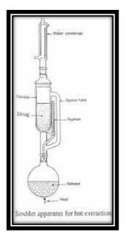
Plant material can be fresh (for example, a plant leaf) or dried. It needs to be crushed, using a pestle and mortar, to provide a greater surface area. The plant material should be sufficient to fill the porous cellulose thimble (in our experiments we use an average of 14 g of thyme in a 25- x 80-mm thimble).
