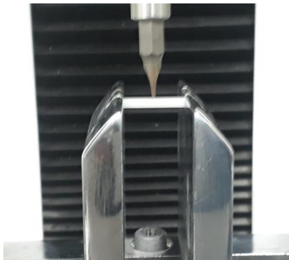
Fig. (1): specimen of exp. PICN material for flexural strength testing mounted on universal testing machine.
