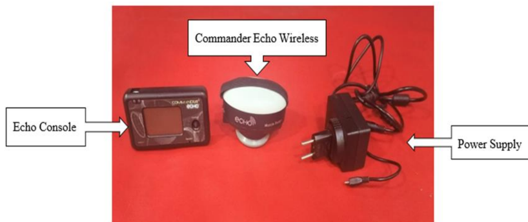
Fig. 1. The components of Muscle strength dynamometer Medical Commander Echo
