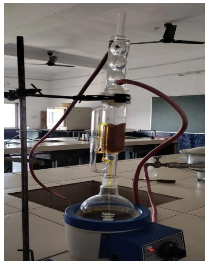
Fig. No. 6.7: Crude drug (turmeric) extraction by soxhlet method
