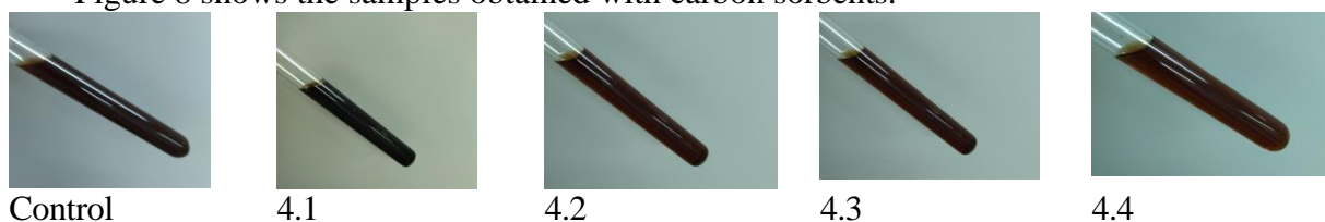
Figure 8 – Wastewater treated with carbon sorbents
