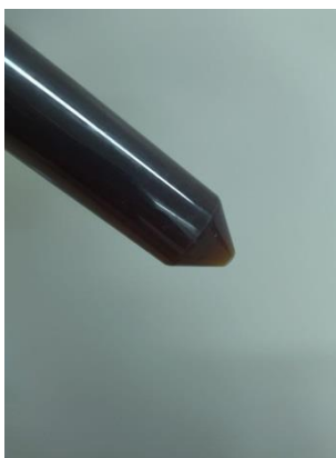
Figure 1 – Aqueous phase of hydrothermal liquefaction of excess activated sludge
