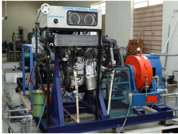
Fig 9 : Test Engine Setup
