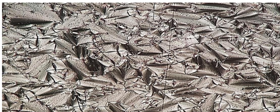
Figure 2. Microphotograph of focal conic texture of SmA mesophase (Series I; n=14 ) at 80
