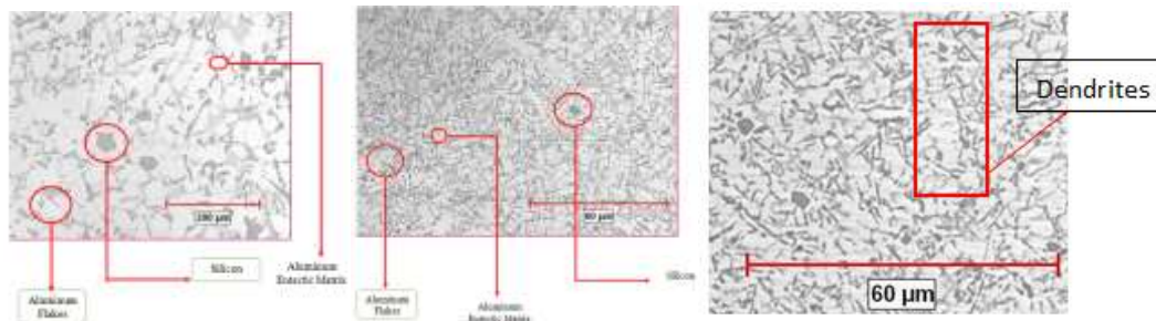
Fig.3. MICROSTRUCTURE OF SAMPLES OF THE DIE AND CORE MOLDS
