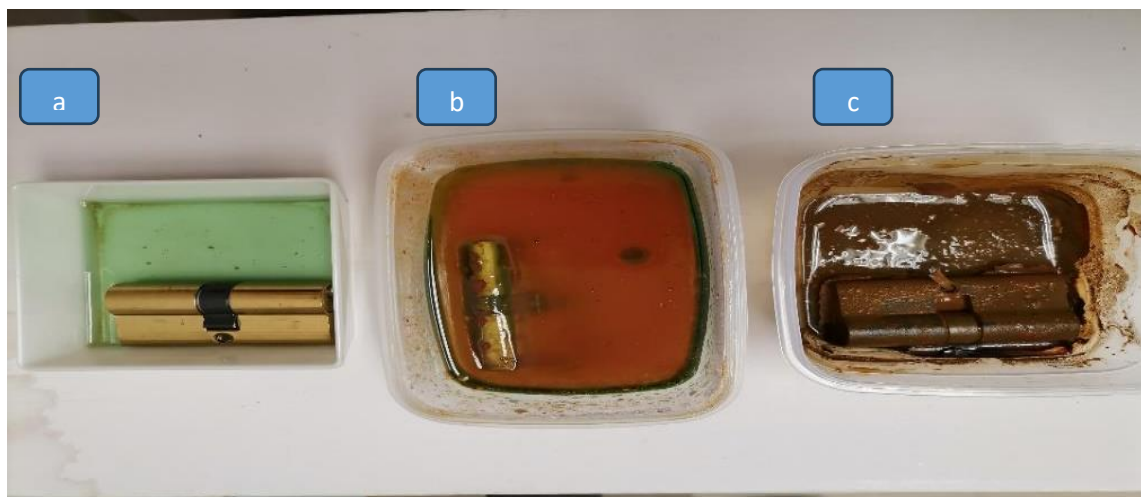
Figure 1. Shows the Jojoba Oil as anti-rust for Metal casting surfaces: a) Surface is better after Jojoba oil coating., b) Rusted positions on the left side and right side without Jojoba oil coating and coated by vegetable oil., c) Surface after is rusted without Jojoba oil coating by water.
