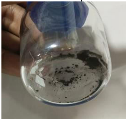
Figure 2: Neem leaves based silver nanoparticles: The dried extract was scraped out and stored in a reagent bottle.
