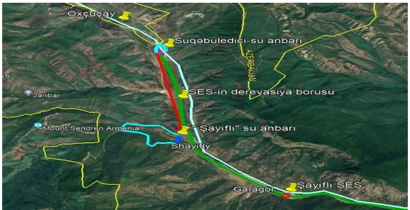
Figure 4. Plan of facilities to be created for ecosystem protection in Okchu River
