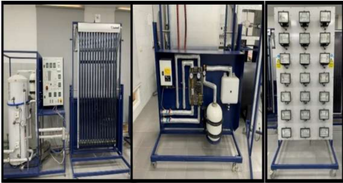
Fig. 15. ETSC complete system [35].
