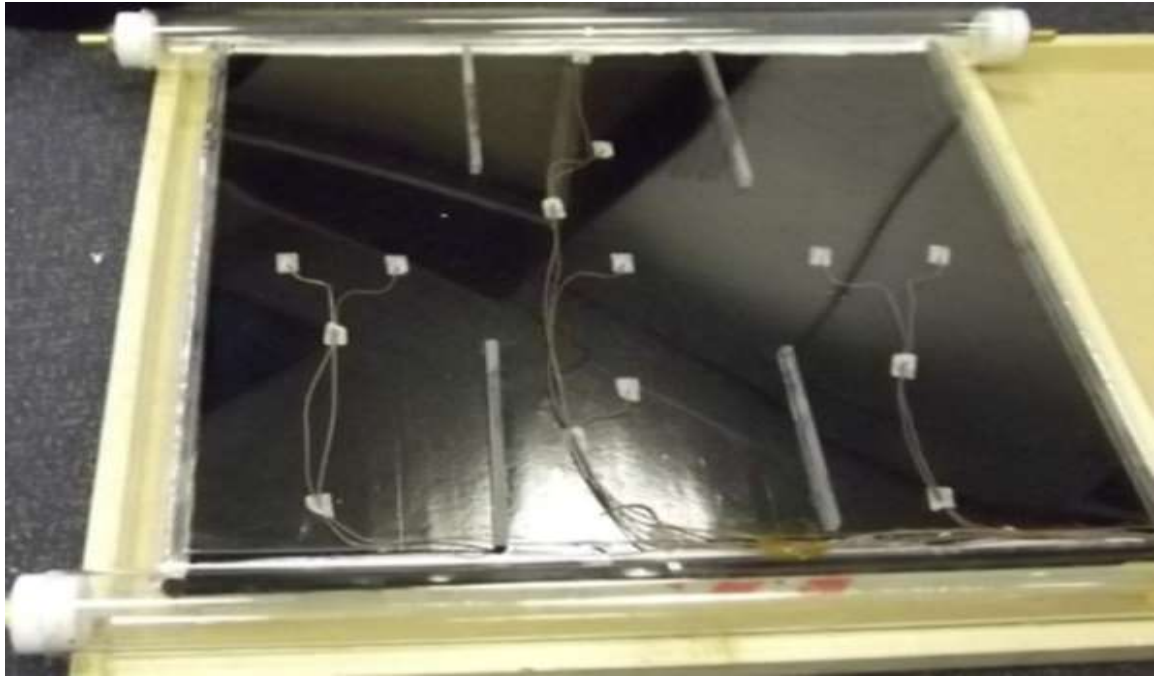
Fig. 1. Proposed PC + CNT solar collector [22].
