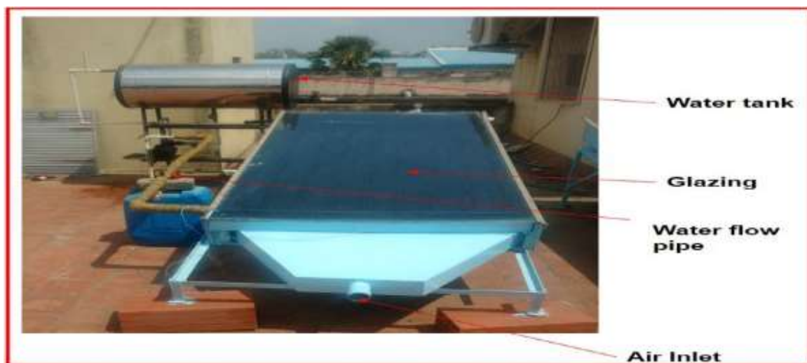
Fig. 4. Pictorial illustration of a hybrid SAH and SWH [25].
