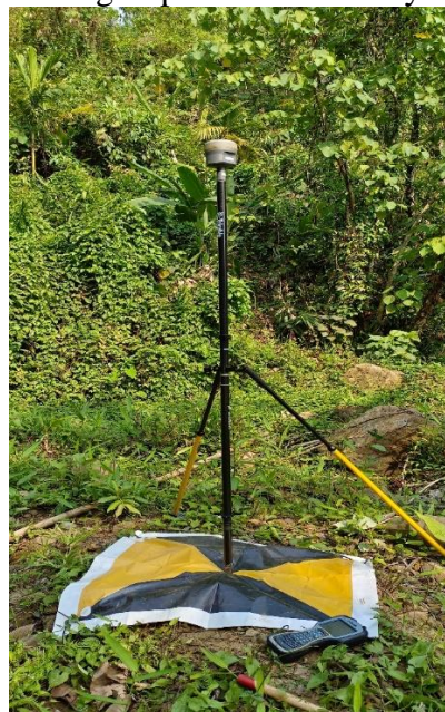
Fig.2: GCP marker & DGPS survey using R12 Aerial Data Collection and Processing
