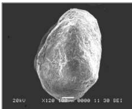
Figure 1211: SEM of coated granule
