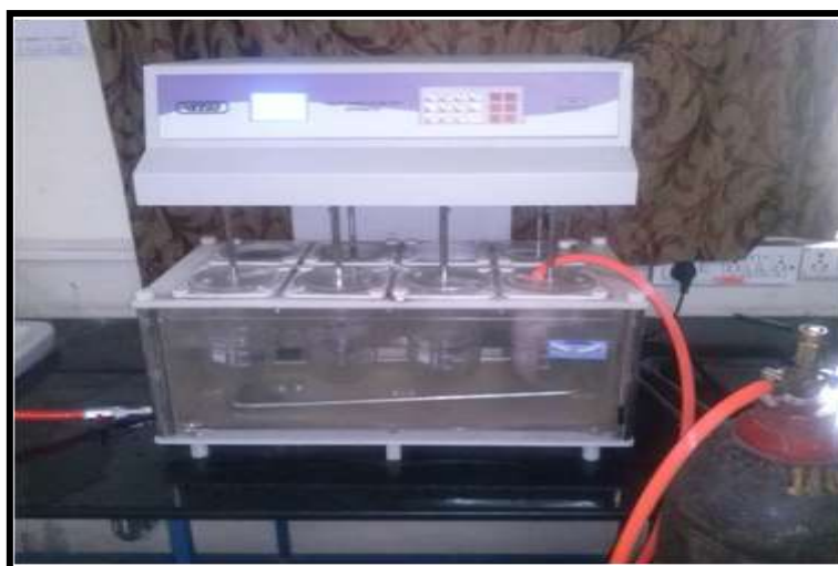
Figure 5: Dissolution apparatus with carbon di oxide supplimentation during content release study
