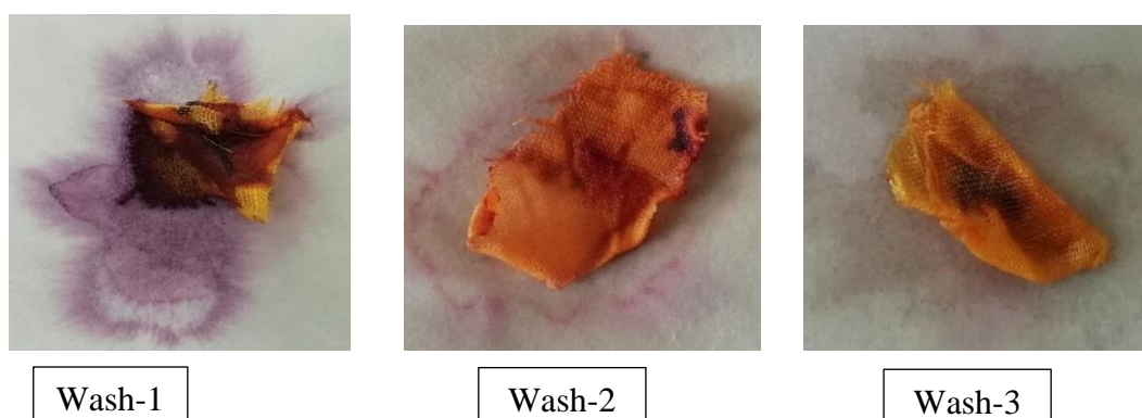
Figure 3: AP test for semen sample (S1) with detergent water washes on cotton fabric
