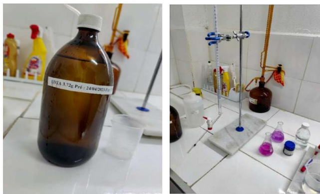
Figure 11: Preparation of Reagents and Solutions for Water Sample Titration.
