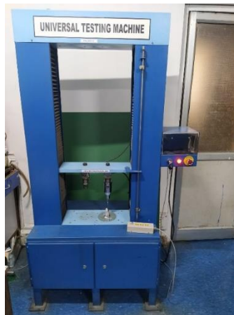
Fig 2:- . Testing of bond strength on sample with universal testing machine.
