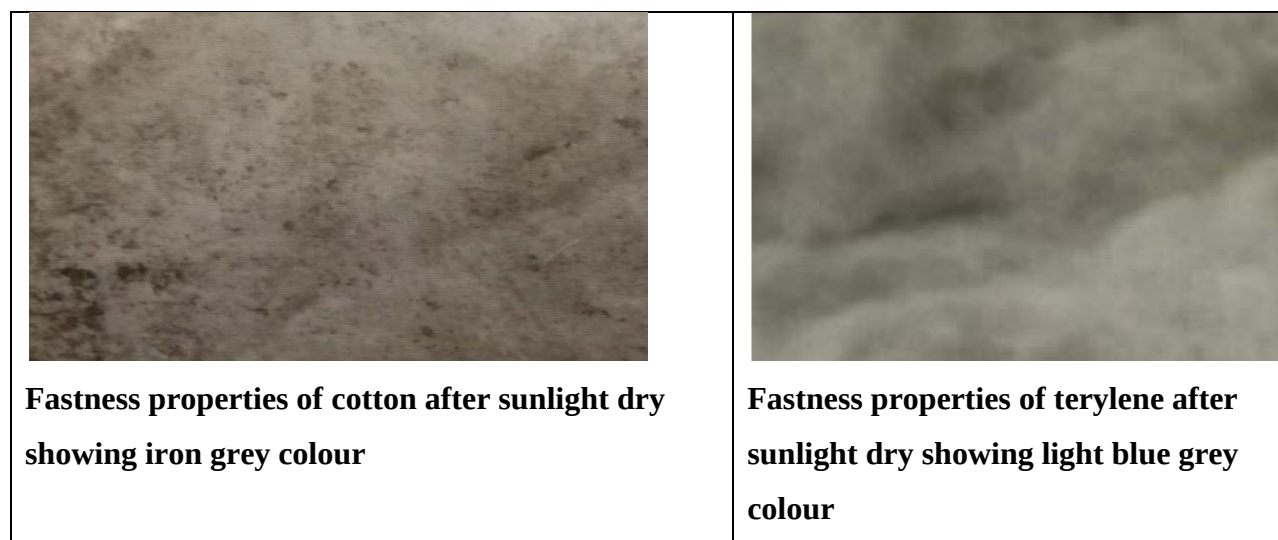
Figure 7: The figure shows the fastness of the colour binding on cotton wool and terylene when the experiment was performed with mordant- Wood ash.
