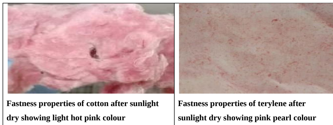
Figure 6: The figure shows the fastness of the colour binding on cotton wool and terylene when the experiment was performed with mordant-Ferrous sulphate.
