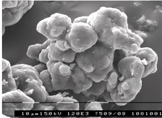
Figure3: Scanning electron photomicrograph of formulation F3 showing population of microspheres.
