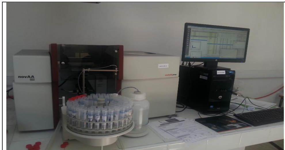
Plate 2: Atomic absorption spectrometer (Faculty of Sciences Kénitra).
