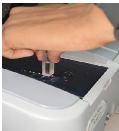
Figure 7: Cuvette with sample in UV-Visible Spectroscopy
